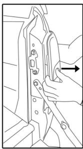
6. Attach damper bracket with the truck using M8 bolts and nut(D)(E). Then put back the rear light.
