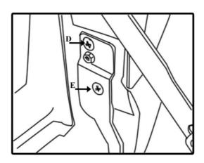
7. Attach damper bracket to the tailgate using original bolts.
