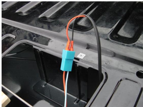
**5) Feed Cable out of the tailgate on Passengers side, Use tubing provided to Protect Cable**
