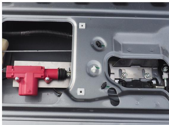
**4) Connect wiring loom to the actuator:**
