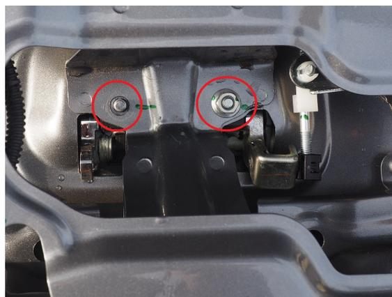
**3) Install the base plate and actuator kit, hold in place by replacing the removed screws from no.2**
