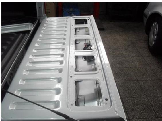
**2) Remove the two screws that hold the tailgate handle into the tailgate**
