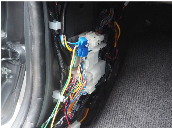
**8) Connect the Central locking kit into the vehicles Central locking Loom**
